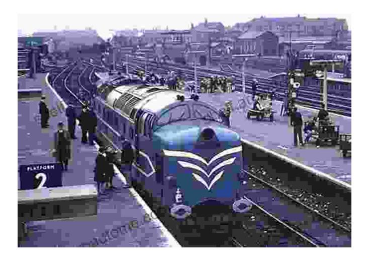
The British Rail Class 55 "Deltic" diesel locomotive, renowned for its speed and power.
