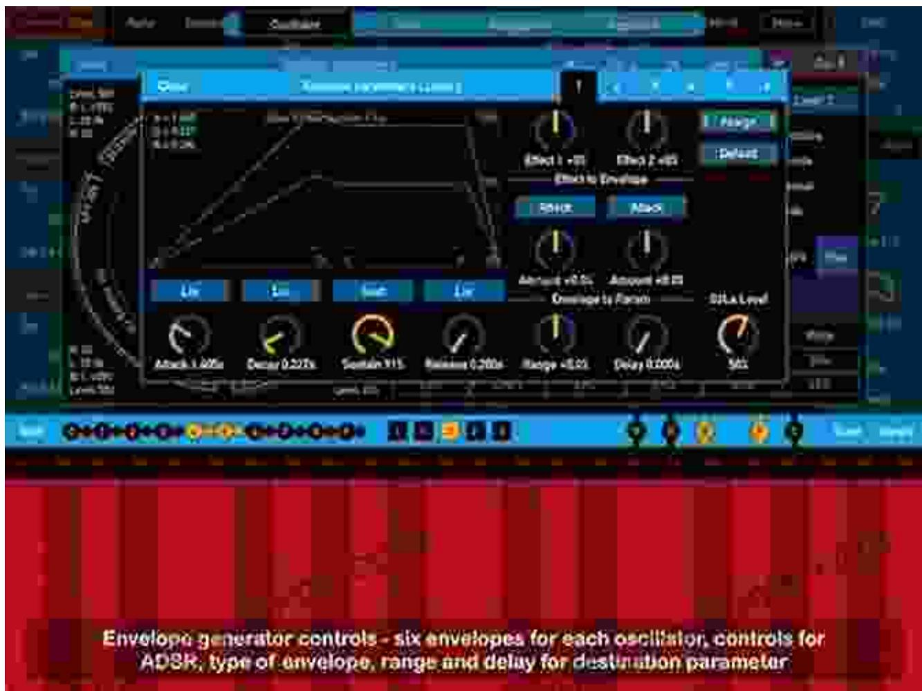
Envelope generator controls - six envelopes for each oscillator, controls for ADSR, type of envelope, range and delay for destination parameter
